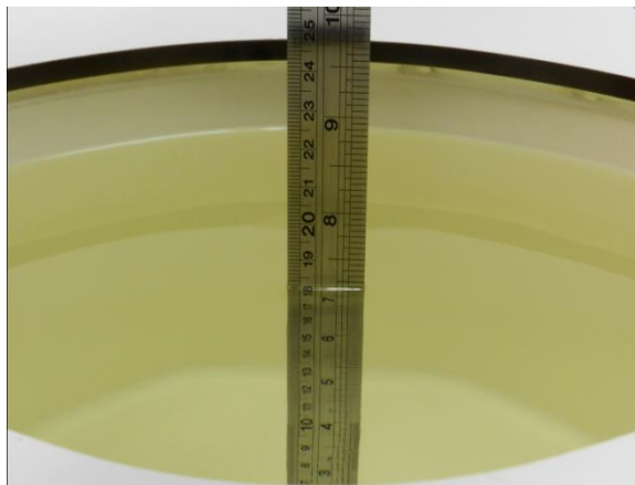
Fig 11.1 Photo of Liquid Height for Body SAR
