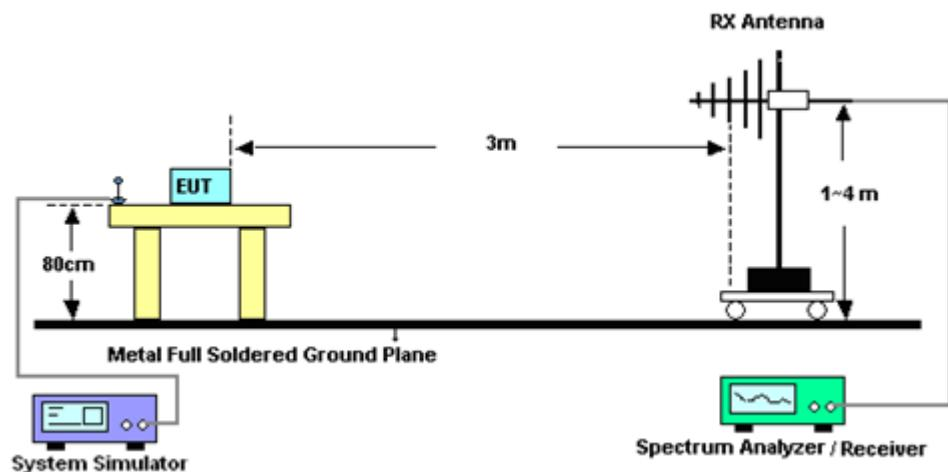
**For radiated test above 1GHz**
