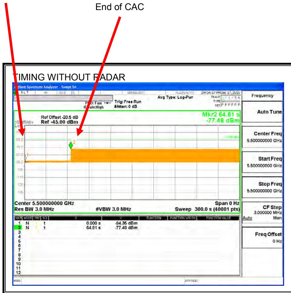
Transmissions begin on channel after completion of the CAC period.
