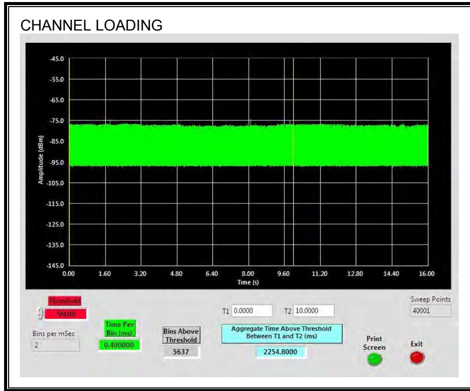
The level of traffic loading on the channel by the EUT is 22.548%
