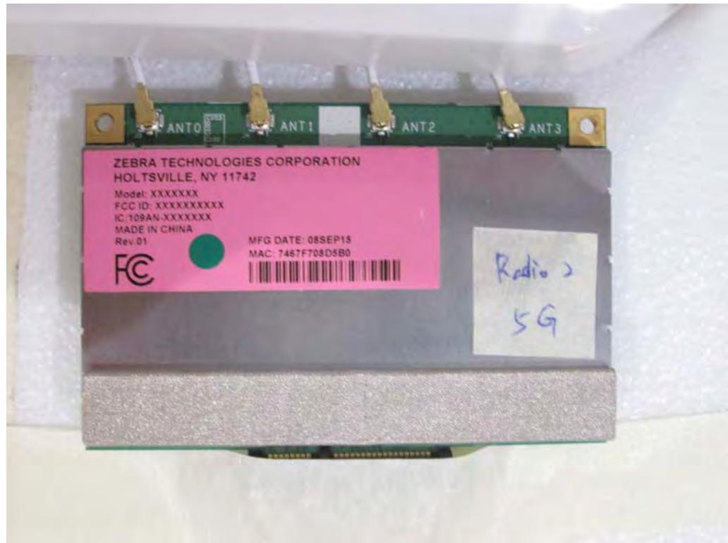
**Mode 1 (Set 1 Dipole antenna / 3.96dBi)**
