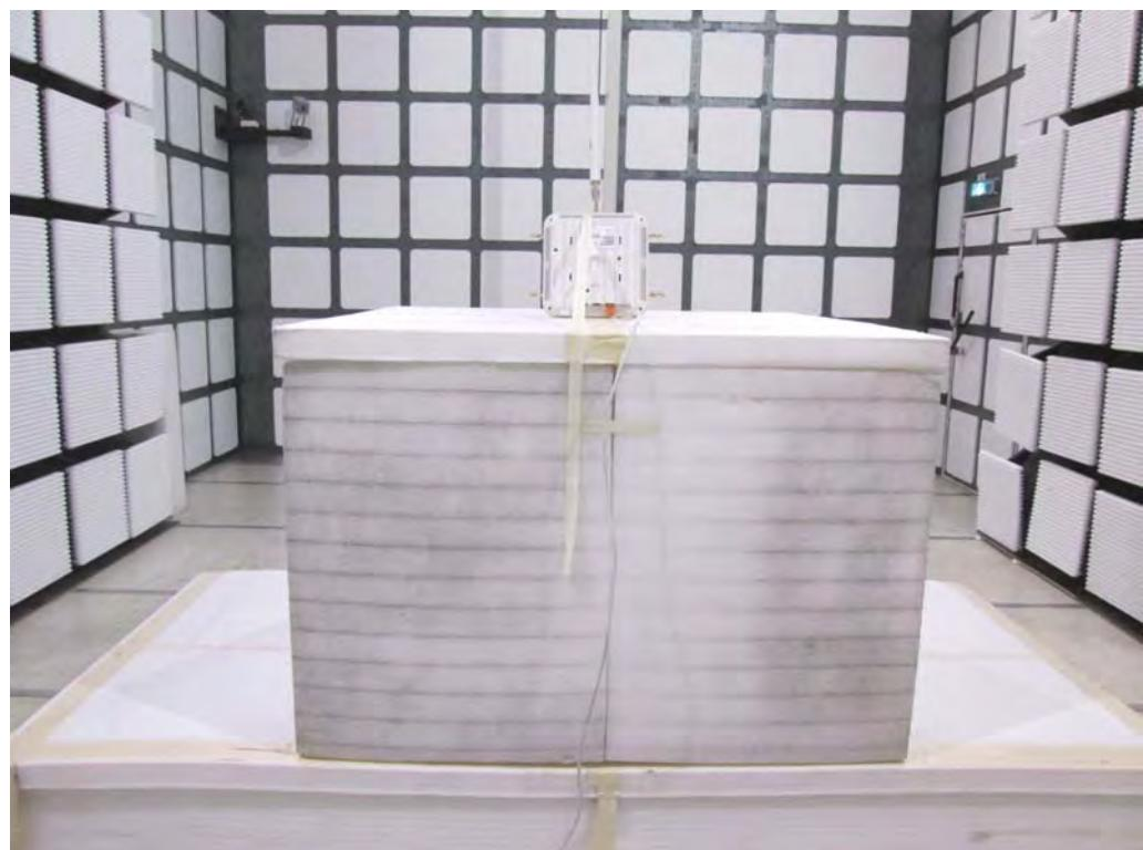
**Test Configuration: Above 1GHz / Mode 2**
