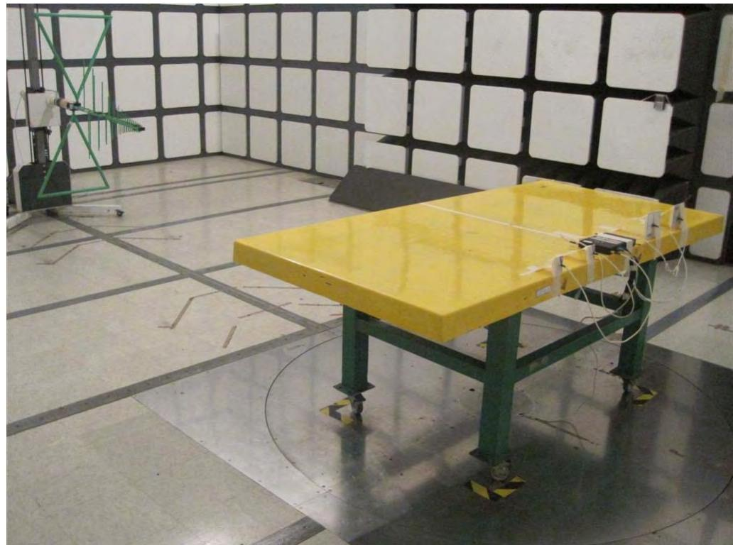
**Test Configuration: 30MHz~1GHz / Power from POE**
