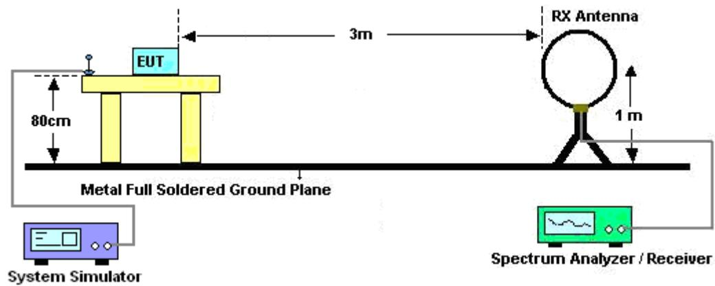
For radiated emissions from 30MHz to 1GHz
