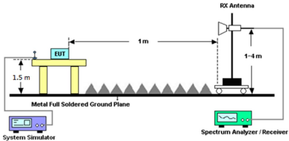
For radiated test above 18GHz
