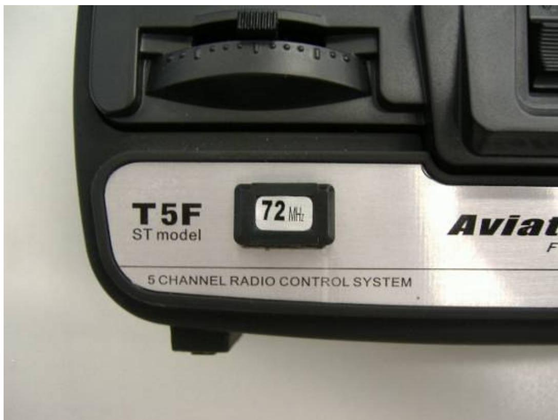
Crystal access panel is permanently glued shut in manufacturing.
