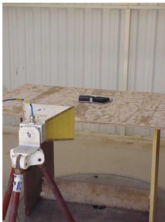
Photo 6. Spurious emissions test setup.
