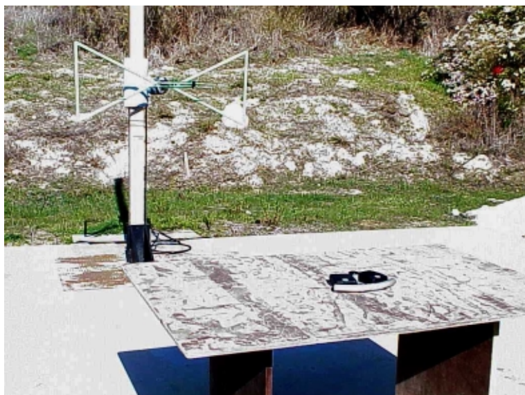
Photo 5. Spurious emissions test setup.
