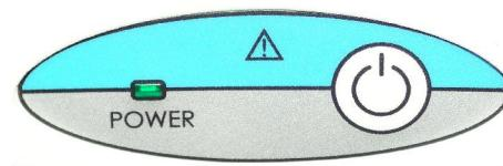
**NOTE:** If the green POWER LED does not go on, you may need to press the MAIN POWER SHUT OFF button on the back of the cart. The system will beep once to indicate power has been turned on.
