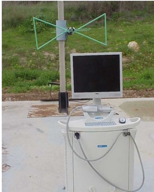
Spurious emissions test setup.
