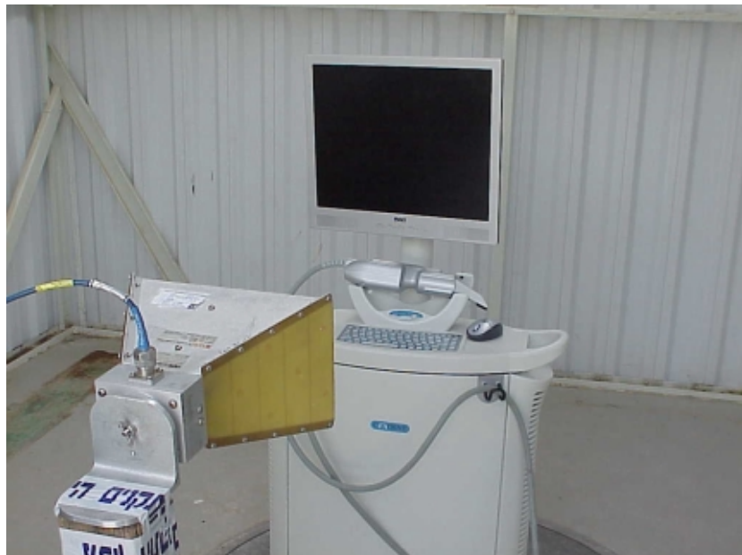
Spurious emissions test setup.
