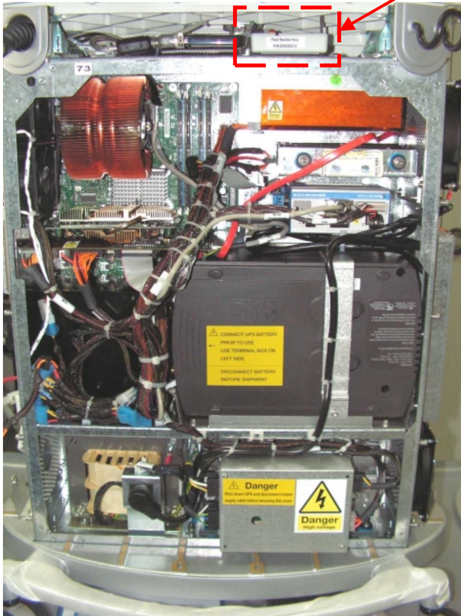
Picture 4. Cart internal view with transceiver location.
