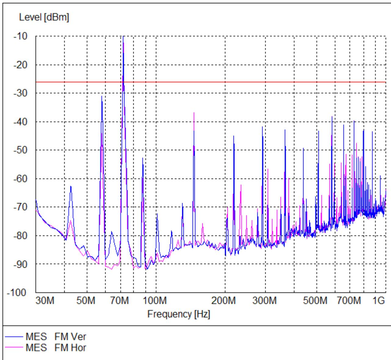
Note: Testing is carried out with 3-orthogonal axis and frequency rang 30MHz to the tenth harmonics. Emissions undetected below the base noise are not reported.
