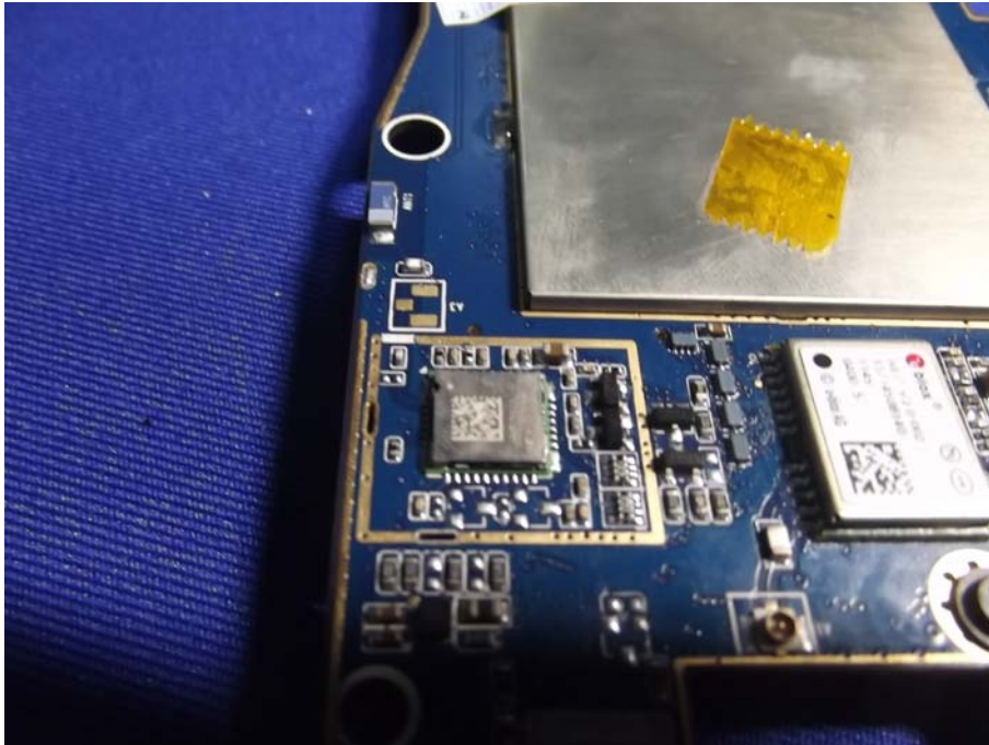
Figure 11 PCB of the WIFI Module View
