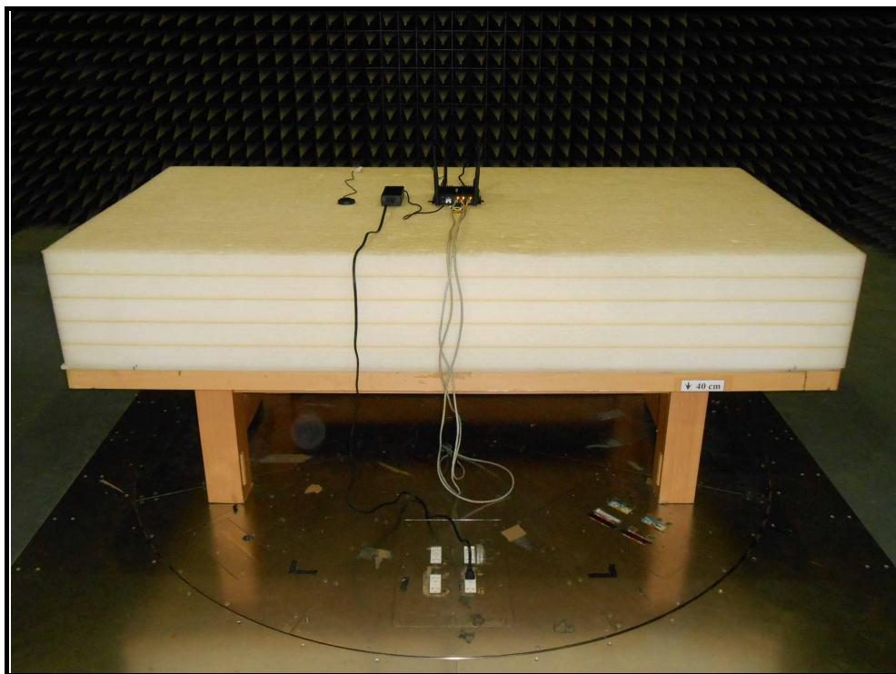
**RADIATED EMISSION TEST (Above 1GHz)**
