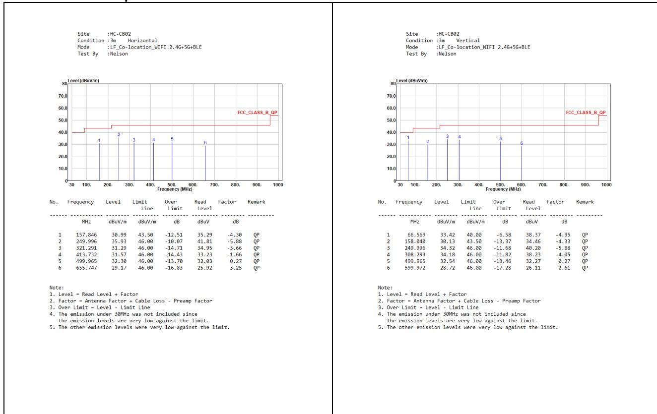
Mode 2: EUT + PoE: WiFi 2.4 GHz + WiFi 5 GHz + Buletooth LE function
