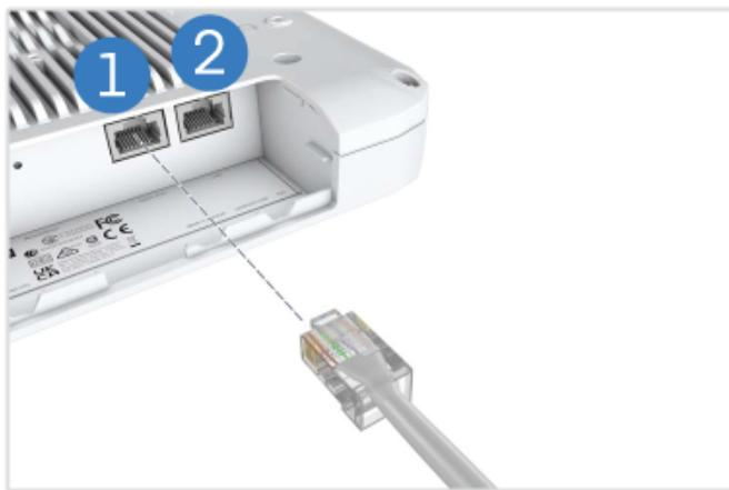
1. Connect a Category 5e or better cable to the Uplink (PoE) 1000BASE-T RJ-45 port. Connect the other end to a PoE source to power to the unit. When power is available, the access point automatically boots up.
