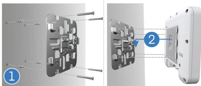
1. At the installation location on the wall, use the metal mounting bracket as a guide to mark four holes for the wall plugs and screws (included in the screw kit). Drill four holes for the anchors, and then insert the anchors. Use a mallet or small hammer to carefully drive the anchors flush with the wall surface. Use the four screws to secure the bracket to the wall.
