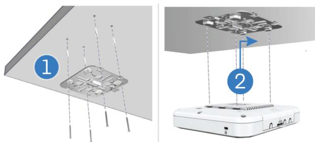
1. At the installation location on the ceiling, use the metal mounting bracket as a guide to mark four holes for the anchors and screws (included in the box). The mounting bracket is not intended for use with drop ceiling T-bars. Drill four holes for the anchors, and then insert the anchors. Use a mallet or small hammer to carefully drive the anchors flush with the ceiling surface. Use the four screws to secure the bracket to the ceiling (screw torque must be less than 6 kgf.cm or .6 Nm).
