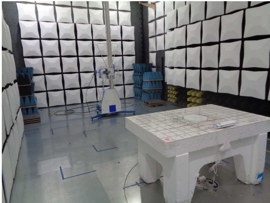
Figure 5: Radiated Spurious Emissions 30 MHz to 1 GHz Back View
