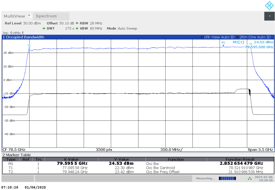
Plot no. 10: 99% OBW, Peak detector, 10 °C
