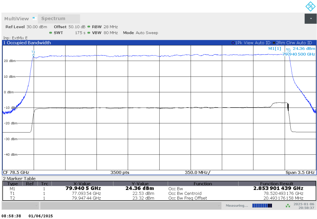
Plot no. 9: 99% OBW, Peak detector, 20 °C, V min
