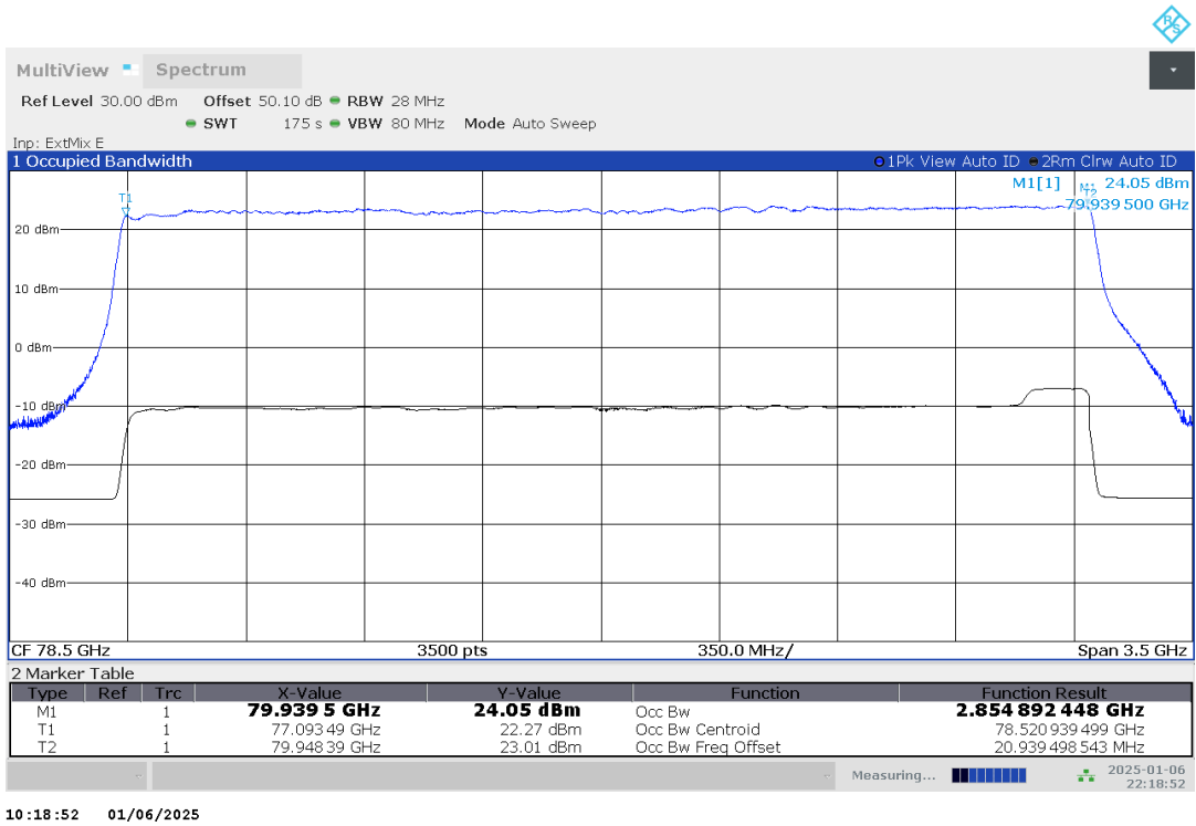
Plot no. 6: 99% OBW, Peak detector, 30 °C
