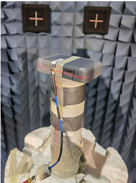
Figure 4 DUT 21234 in free space passive measurement
