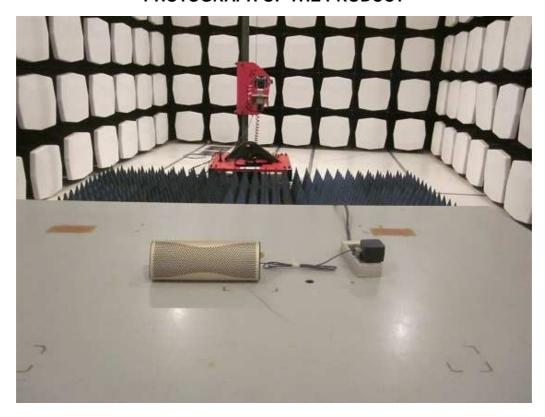
**MEASUREMENT OF CONDUCTED EMISSION TEST SET UP**
