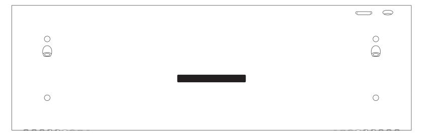
Recess for serial label: Laser etch/CNC: 0.15 Depth
