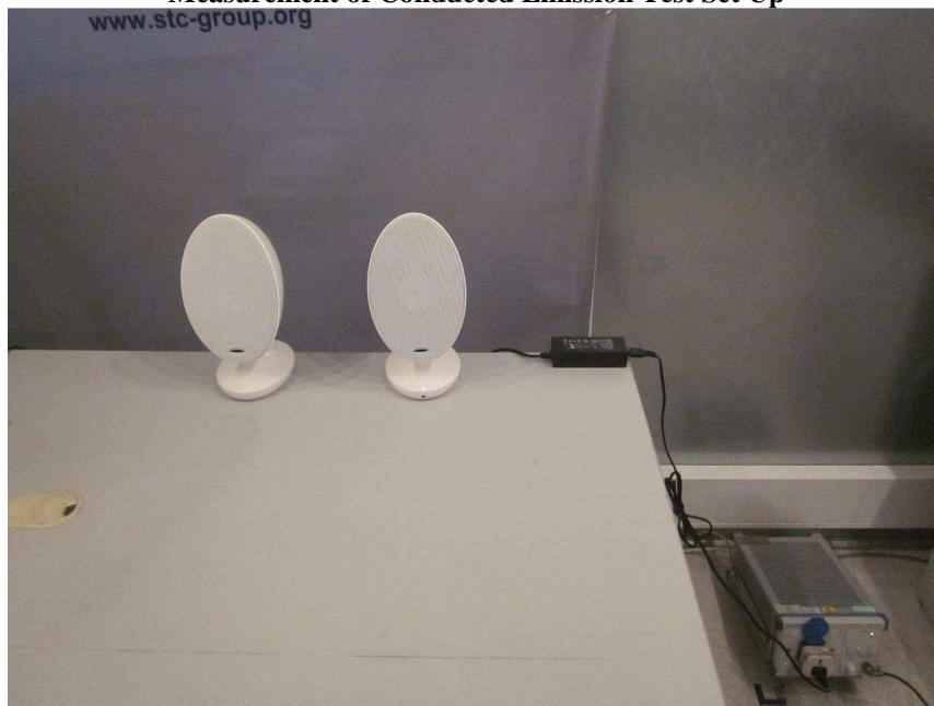
Measurement of Conducted Emission Test Set Up
