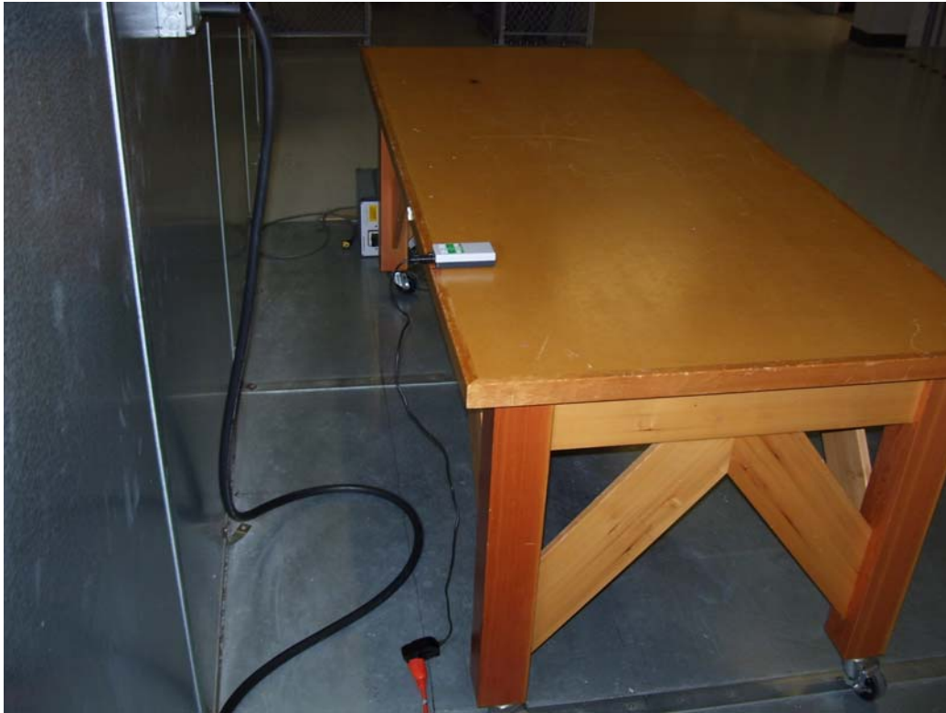
Figure 7 - Conducted Emissions Test Setup
