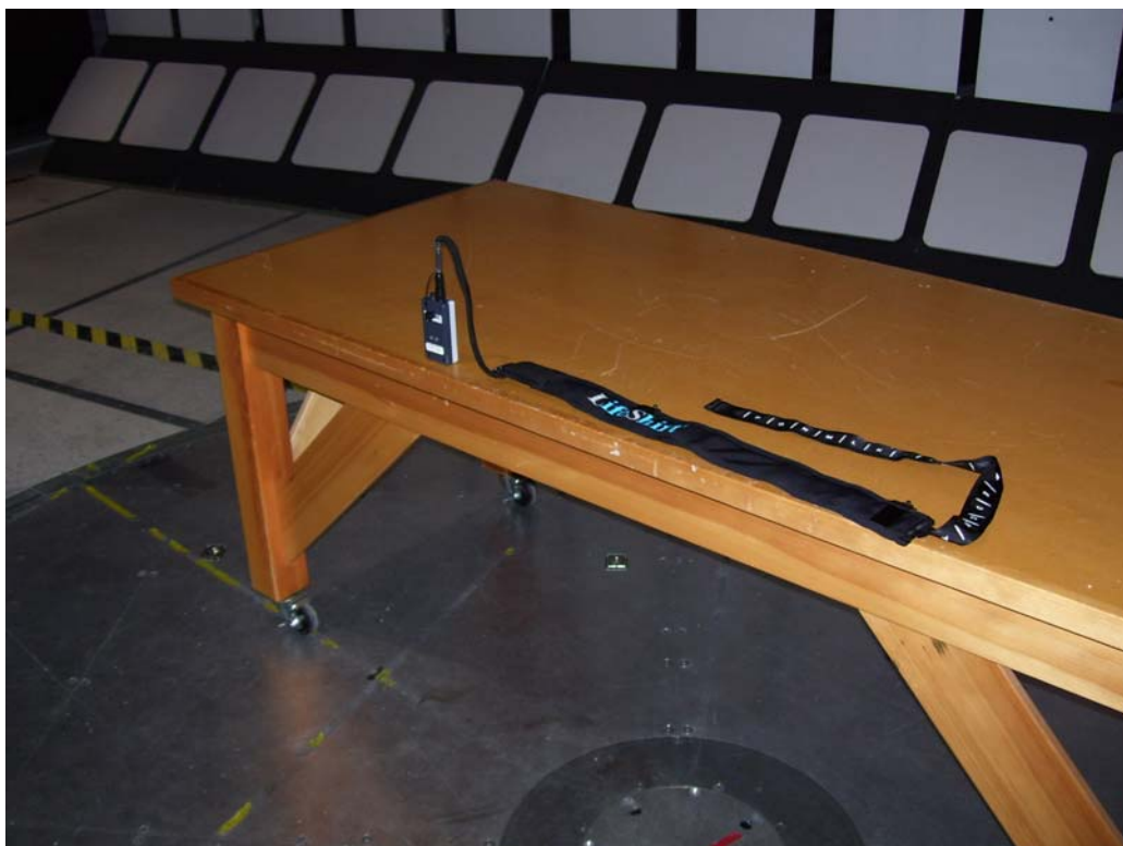
Figure 6 - Radiated Emissions Test Setup, Upright Configuration
