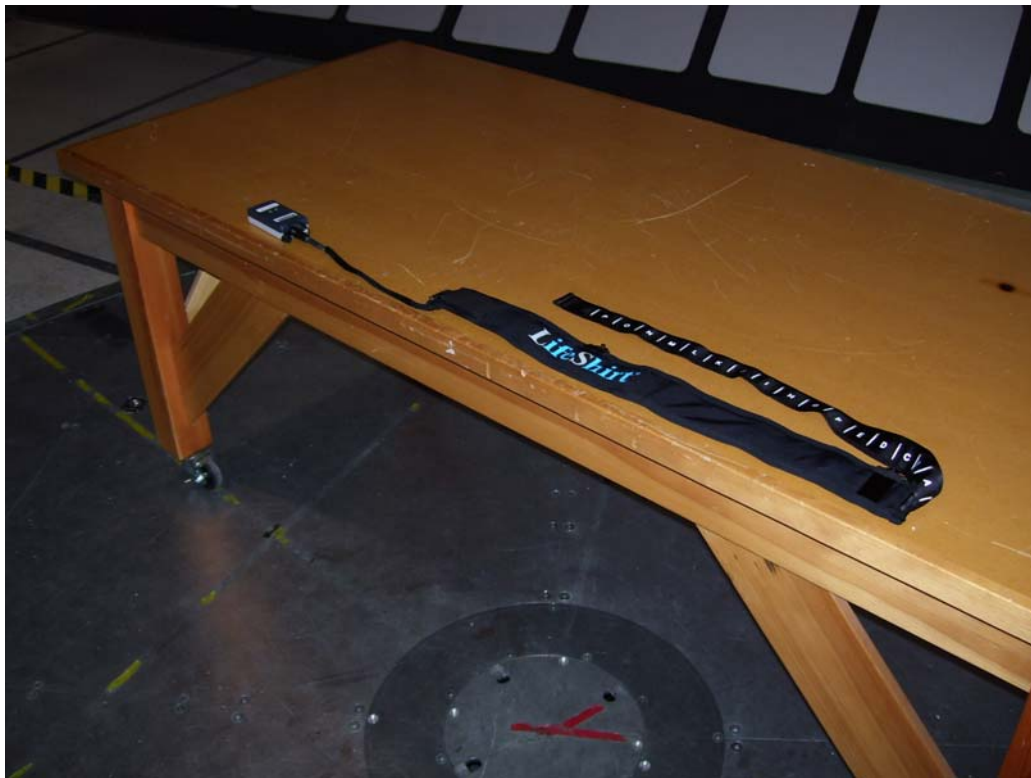
Figure 5 - Radiated Emissions Test Setup, Sideways Configuration
