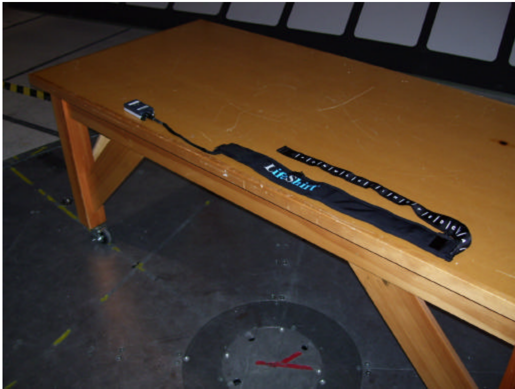
Figure 8 - Radiated Emissions Test Setup, Sideways Configuration
