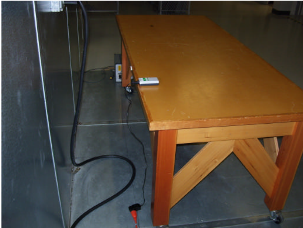
Figure 10 - Conducted Emissions Test Setup
