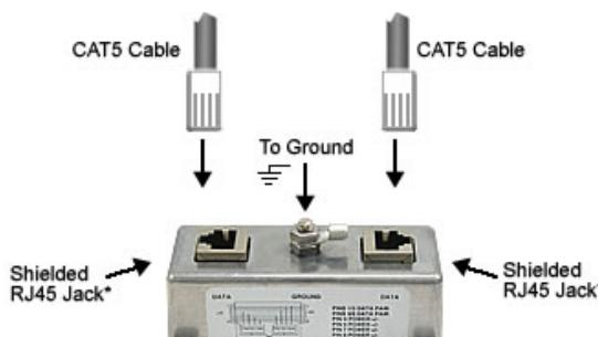
\*Unit provides protection to both jacks equally.
