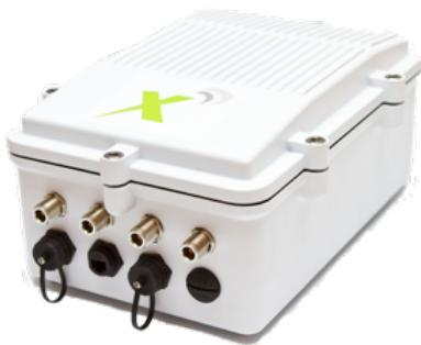
The Acurix Networks X3-N-XX intelligent wireless node delivers a whopping 900 Mbps of connectivity supporting 3 x 300 Mbps links for backhaul and access in any mix of point-to-point, point-to-multipoint, mesh and infrastructure-mesh configurations. Each of the three radios is capable of supporting links up to 300 Mbps and can do 20 or 40 MHz channels.
