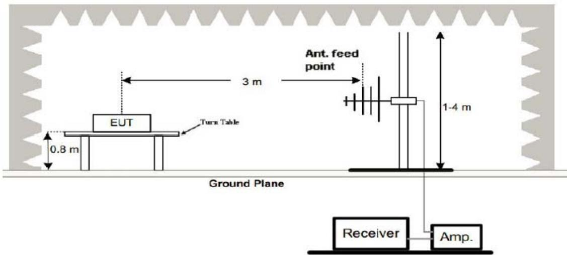
(3) Radiated Emission Test-Up Frequency Above 1GHz
