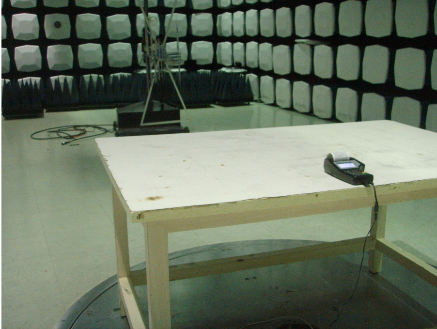
Radiation Emission Test – Front View
