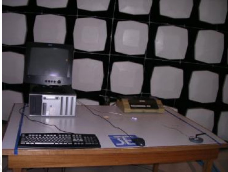
Measurement of Radiated Emission Test Set Up
