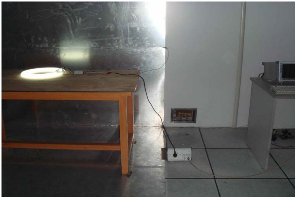
Conducted Emission Test View for EBU3240MA (72W)
