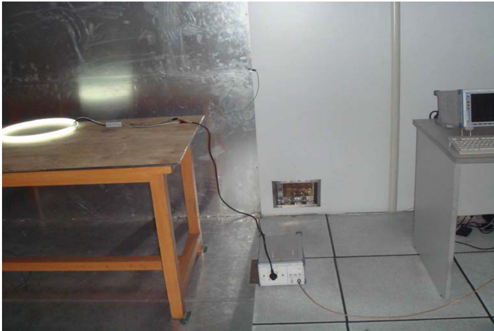
Conducted Emission Test View for EBU2232MA (54W)
