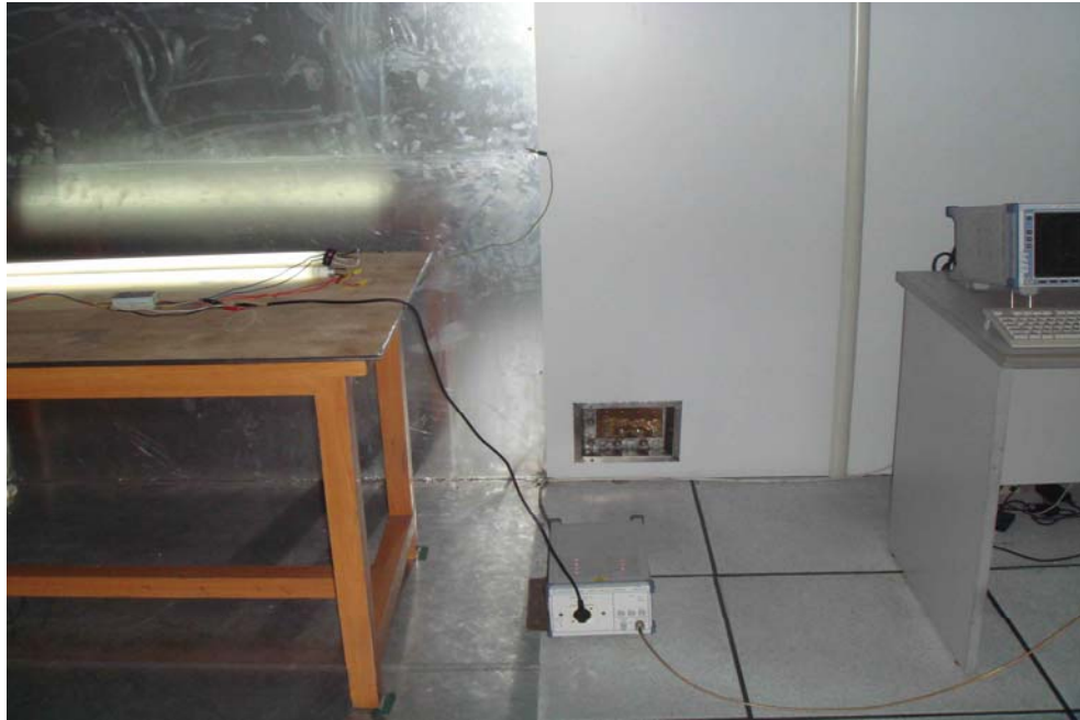
Conducted Emission Test View for EBU3240MA (72W)
