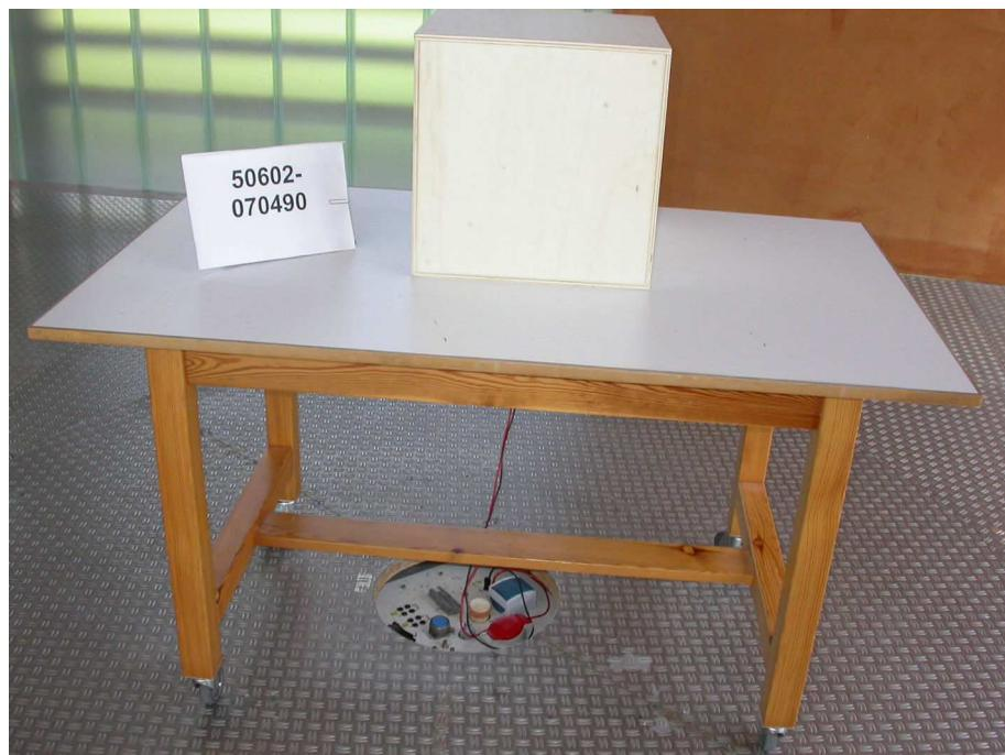
**Test setup for radiated emission measurement
