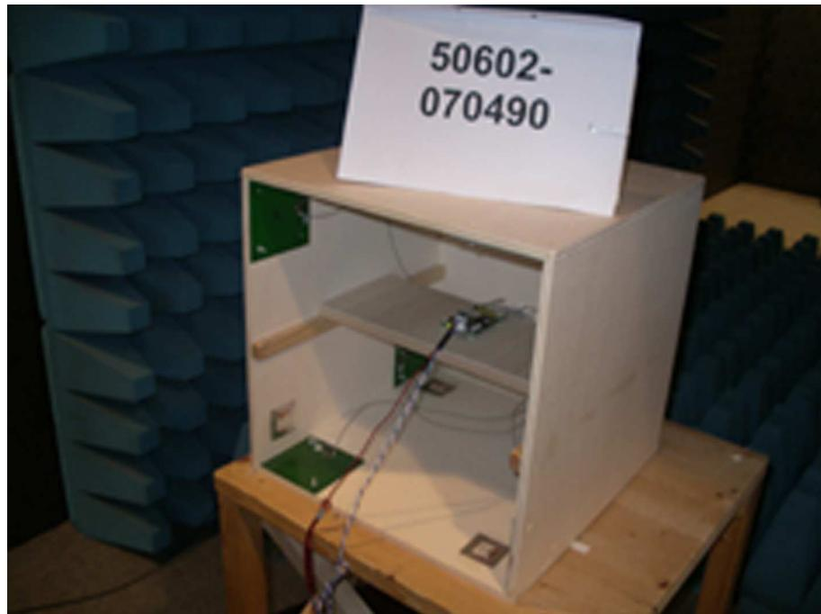
**Test setup for radiated emission measurement
