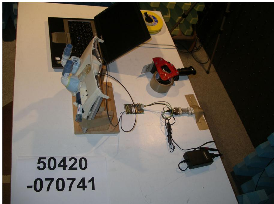
**Test setup for radiated emission measurement
