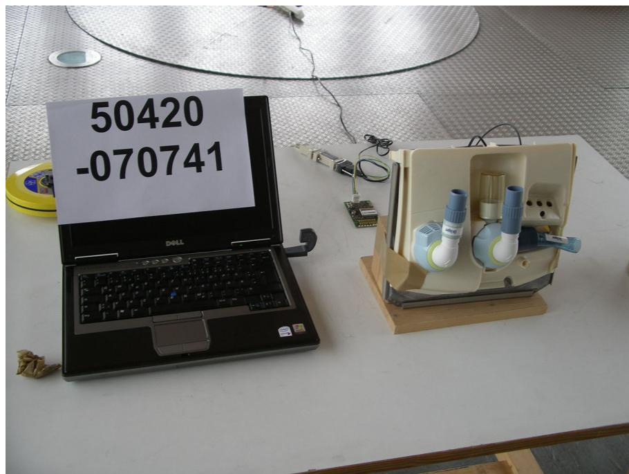
**Test setup for radiated emission measurement
