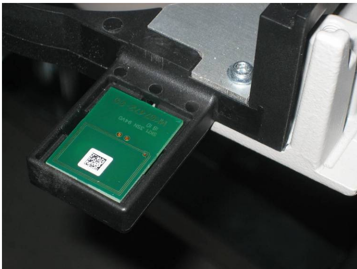
Figure 29: Placement of Antenna Breath Ex, MK07477 in A500
