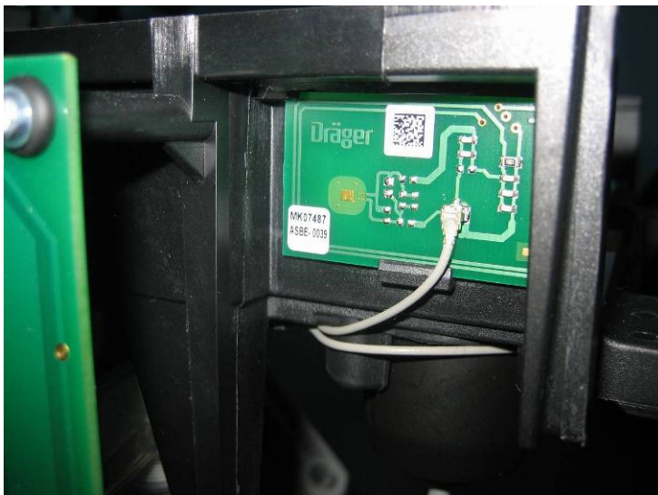
Figure 27: Placement of Antenna Flow Ex, MK07487, in A500
