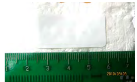
Transponder (Tag), fixed on Styrofoam
