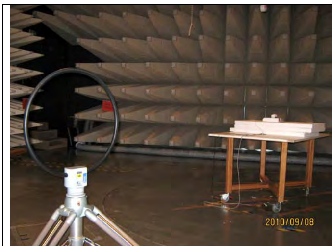
Radiated emissions measurement at 3 m distance
