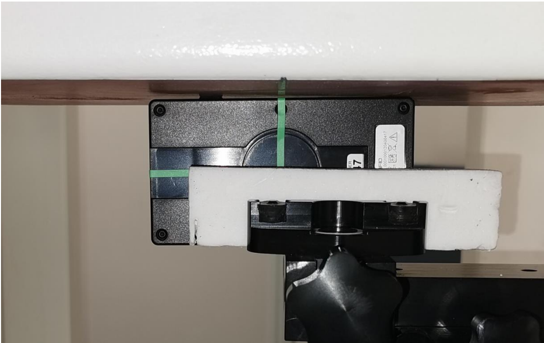
Left test position, Extremity 0mm separation distance
