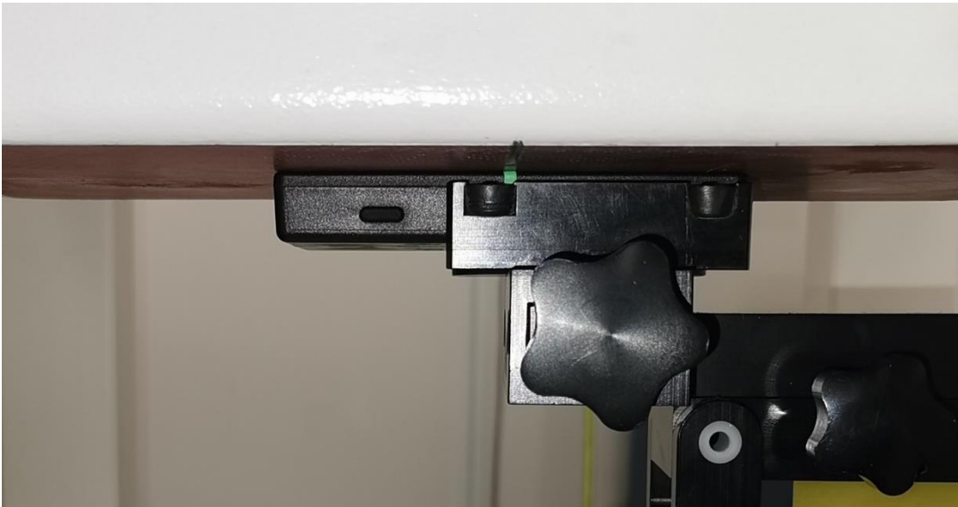
Back test position, Extremity 0mm separation distance
