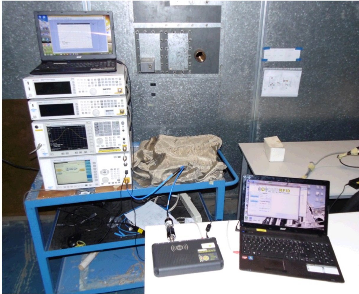
Fig. 8.5 Conducted Transmission Test Set-up
