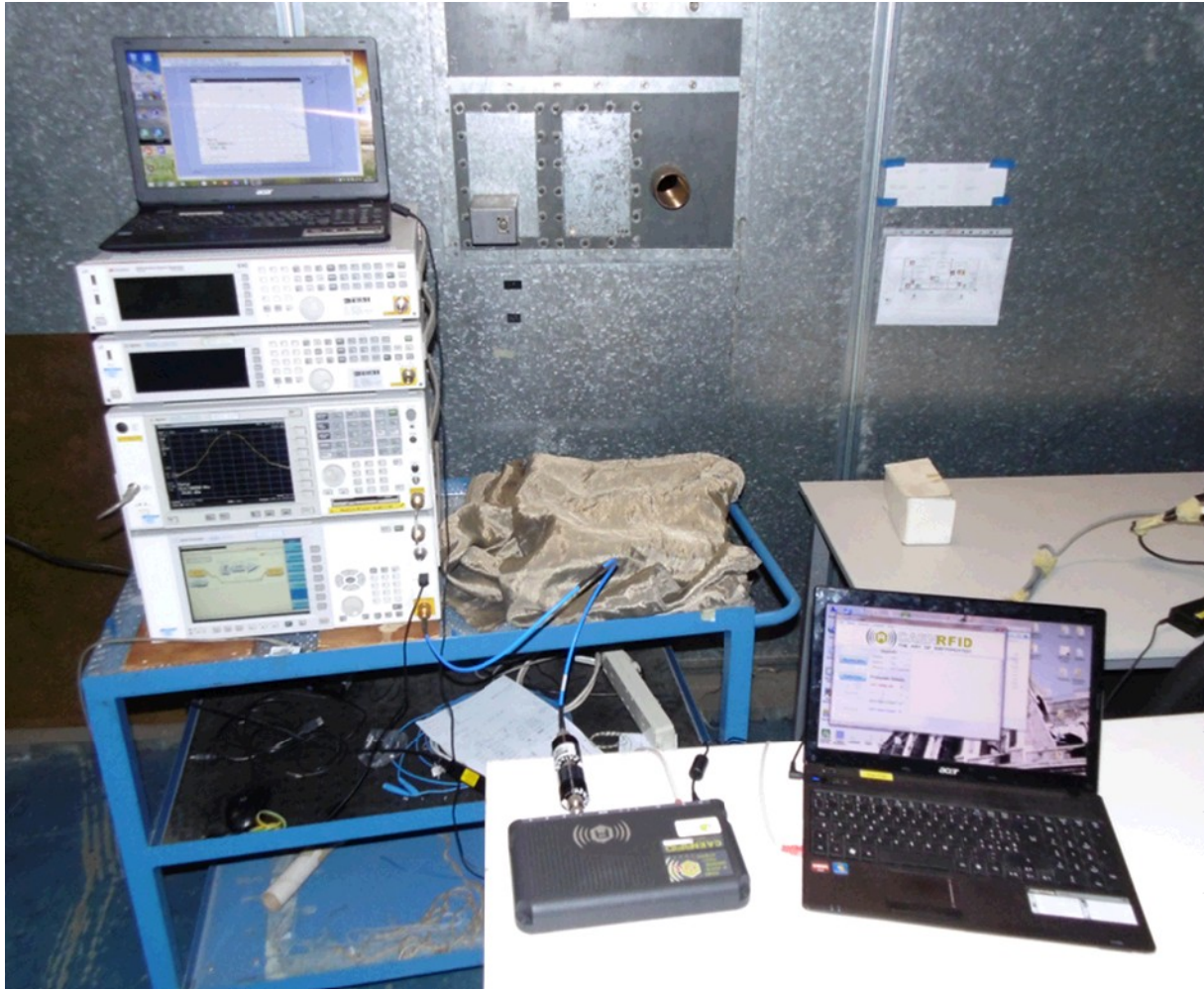
Fig. 8.5 Conducted Transmission Test Set-up
