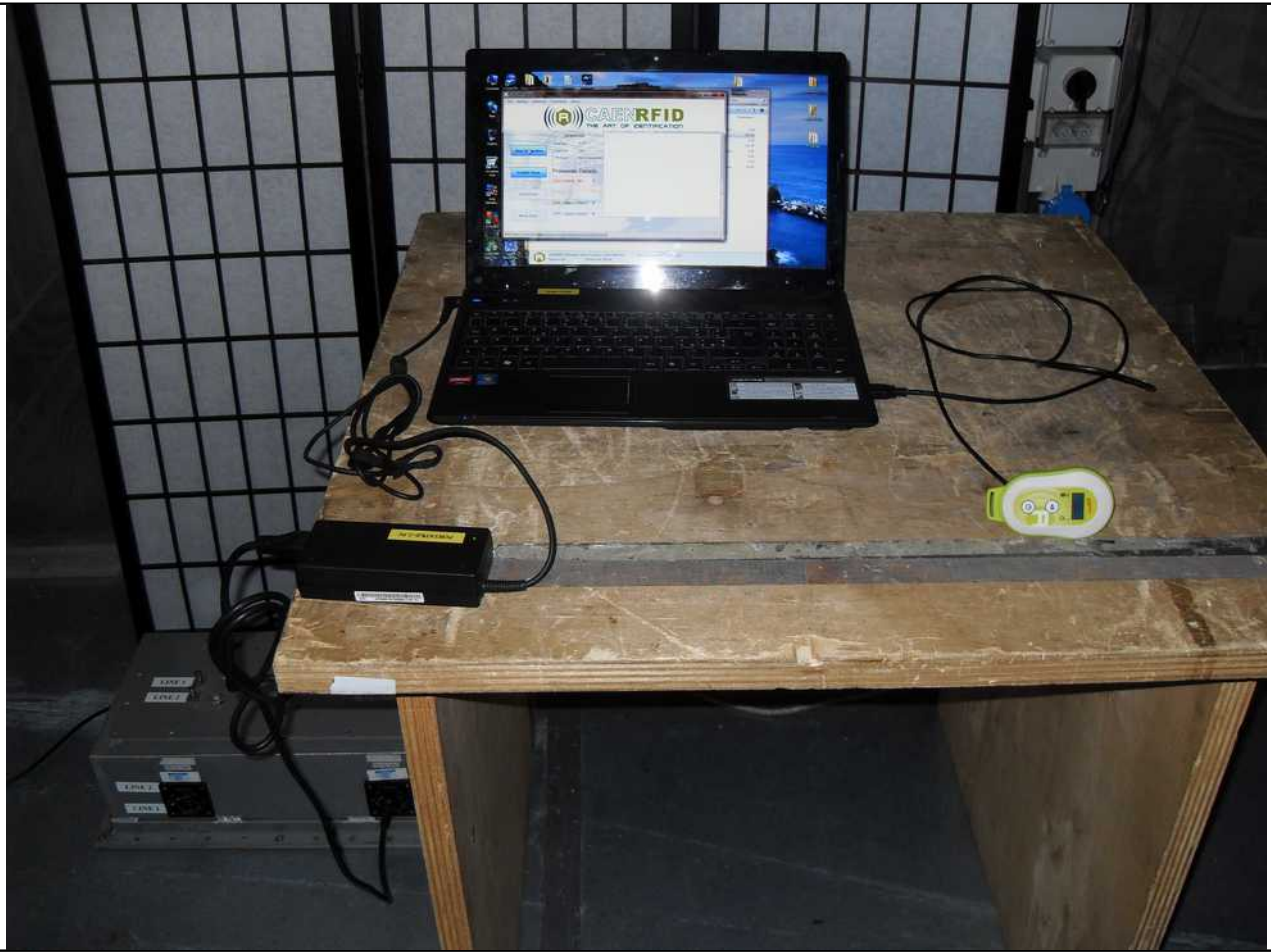
Fig. 6.1 Conducted Emissions Test Set-up
