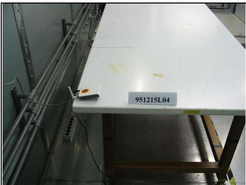
RADIATED EMISSION TEST (Test Mode A)
