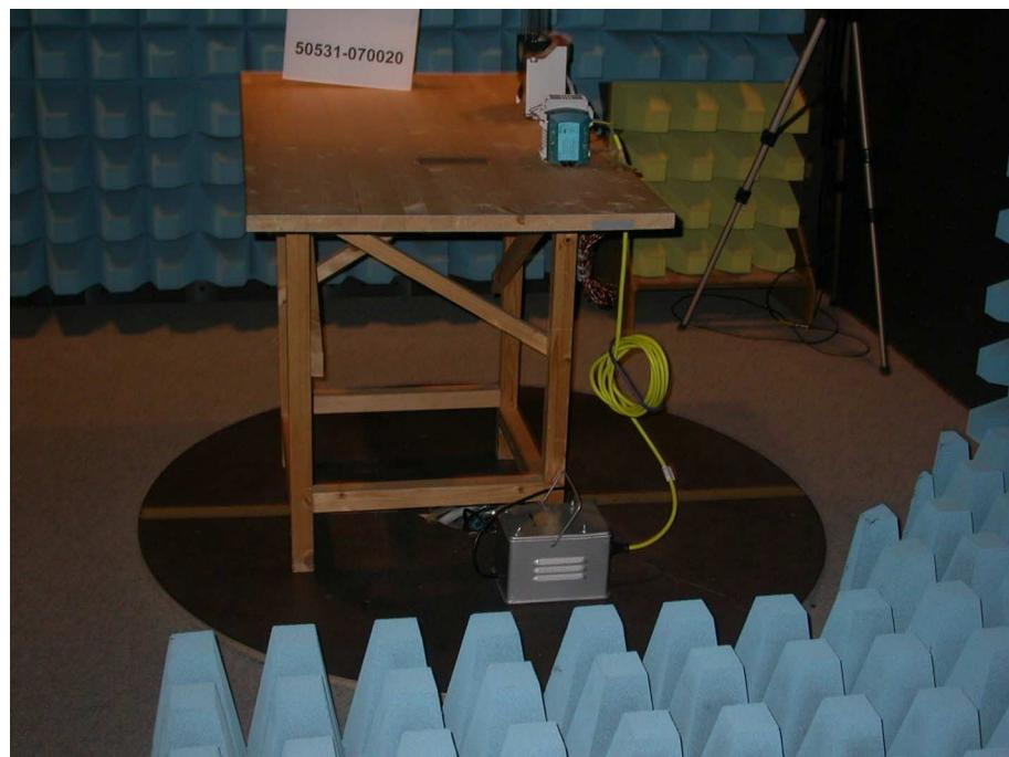
**Test setup for radiated emission measurement
