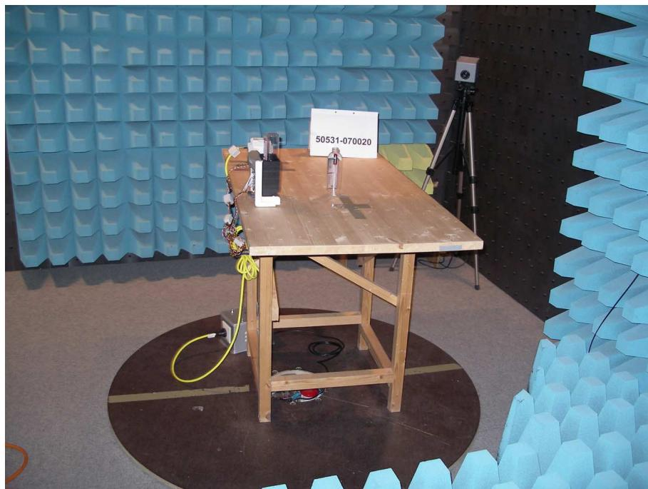
**Test setup for radiated emission measurement
