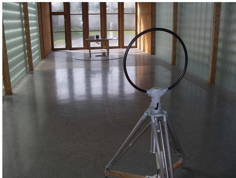
**Test setup for radiated emission measurement
