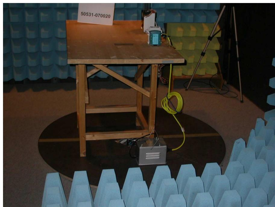
**Test setup for radiated emission measurement
