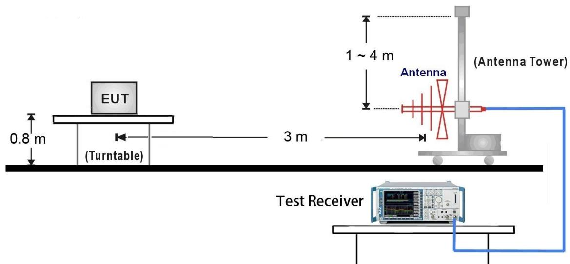
1GHz ~ 18GHz Test Setup:
