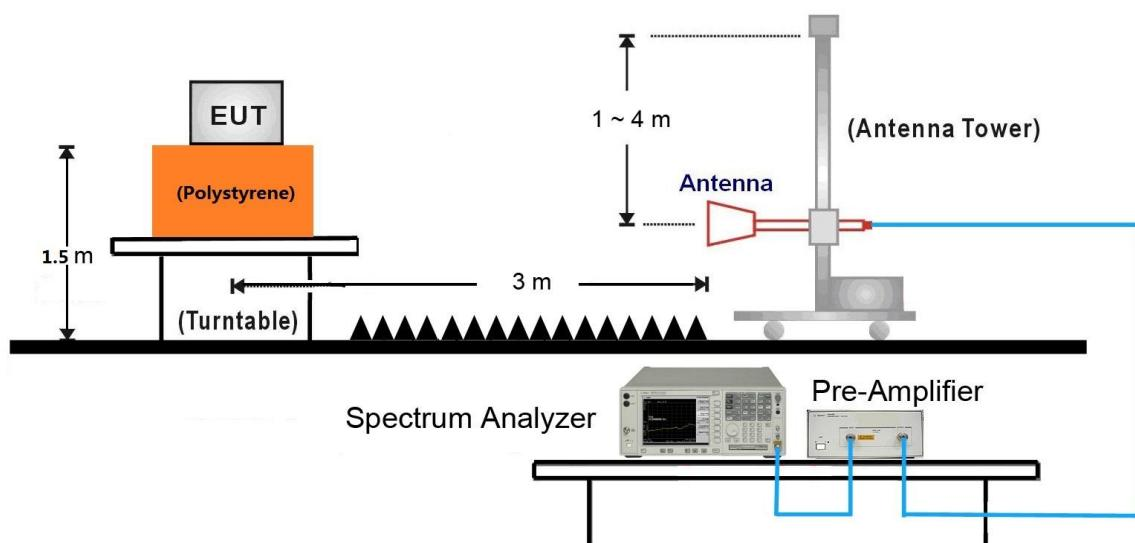
18GHz ~25GHz Test Setup:
