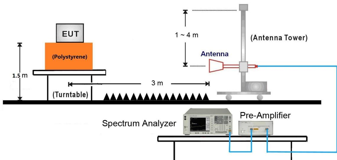
18GHz ~25GHz Test Setup:
