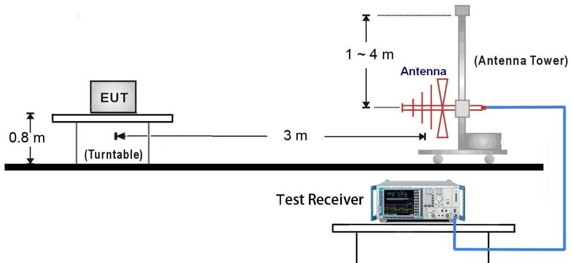
1GHz ~ 18GHz Test Setup:
