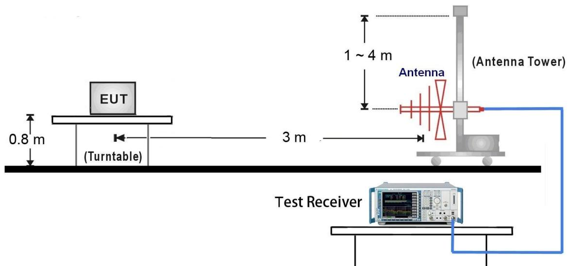
1GHz ~ 18GHz Test Setup:
