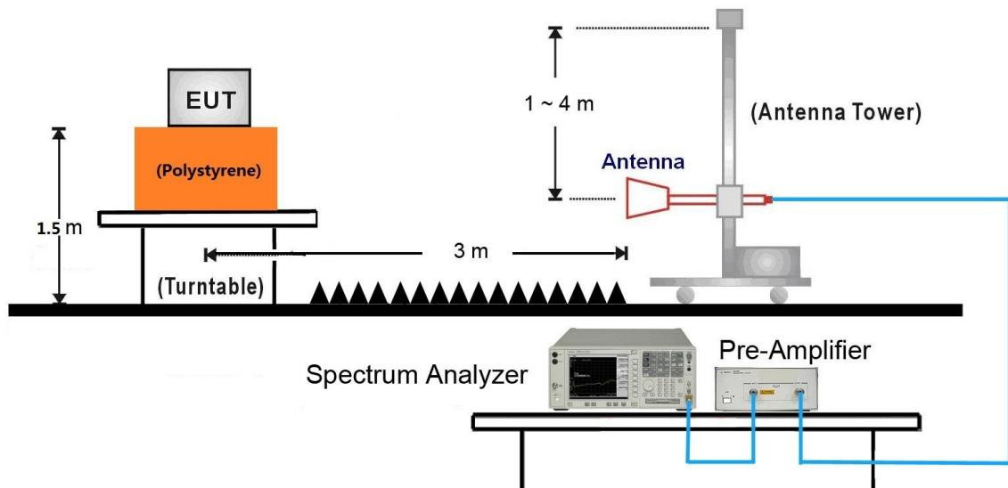
18GHz ~25GHz Test Setup:
