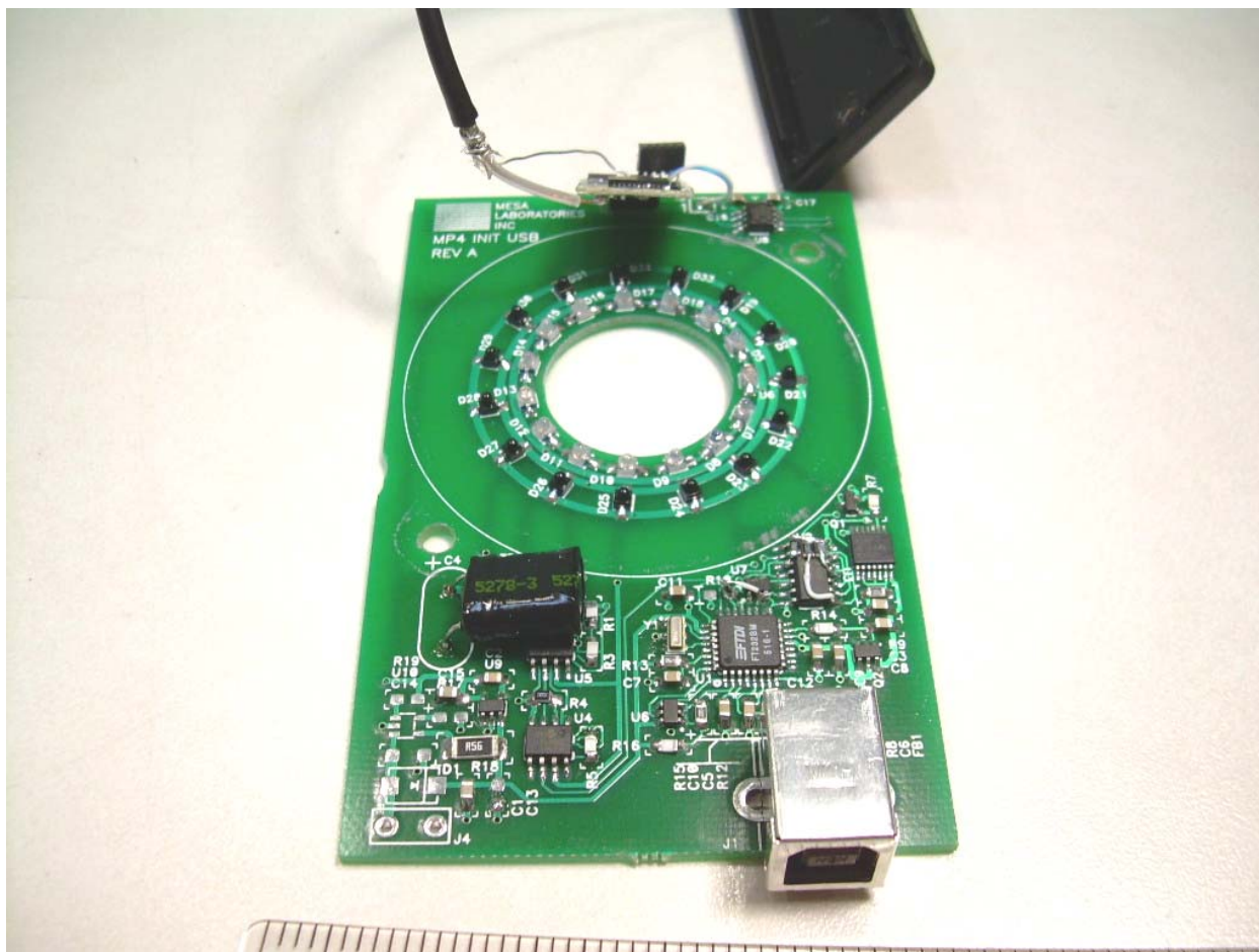
View of the Component Side of the MPRF-H PCB with Mirror Removed
