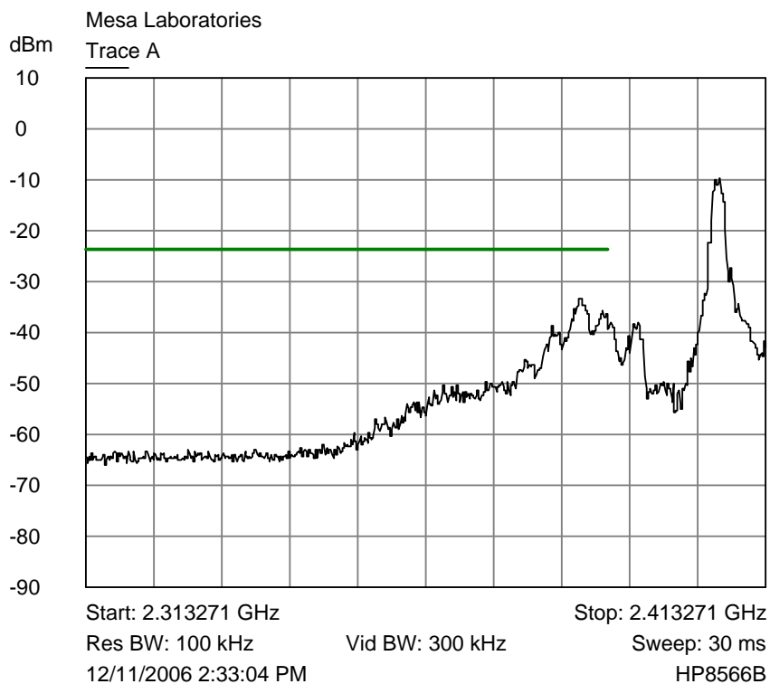
Trace A Ch 0 band edge plot
