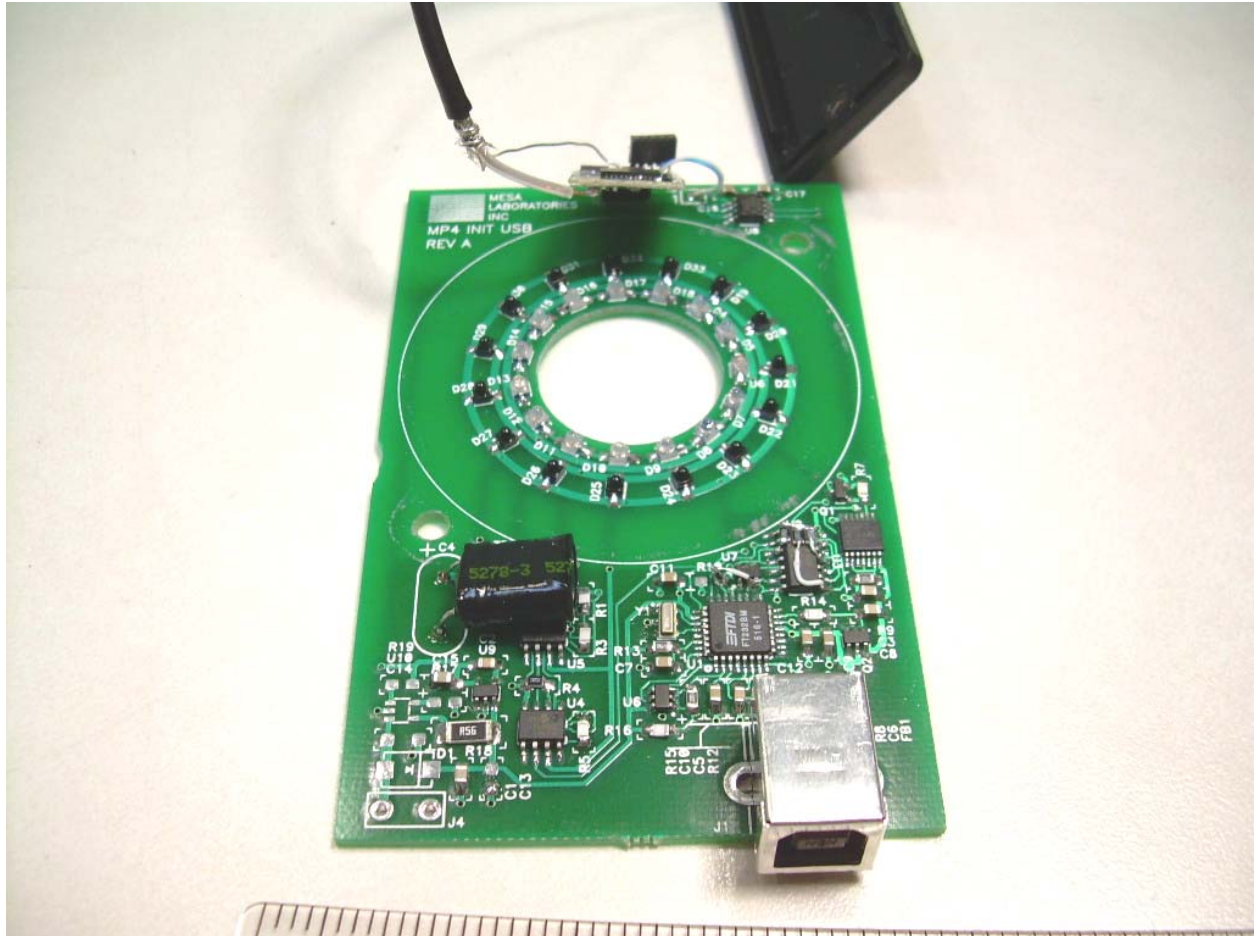
Photograph 8 -View of the Component Side of the MPRF-H PCB with Mirror Removed
