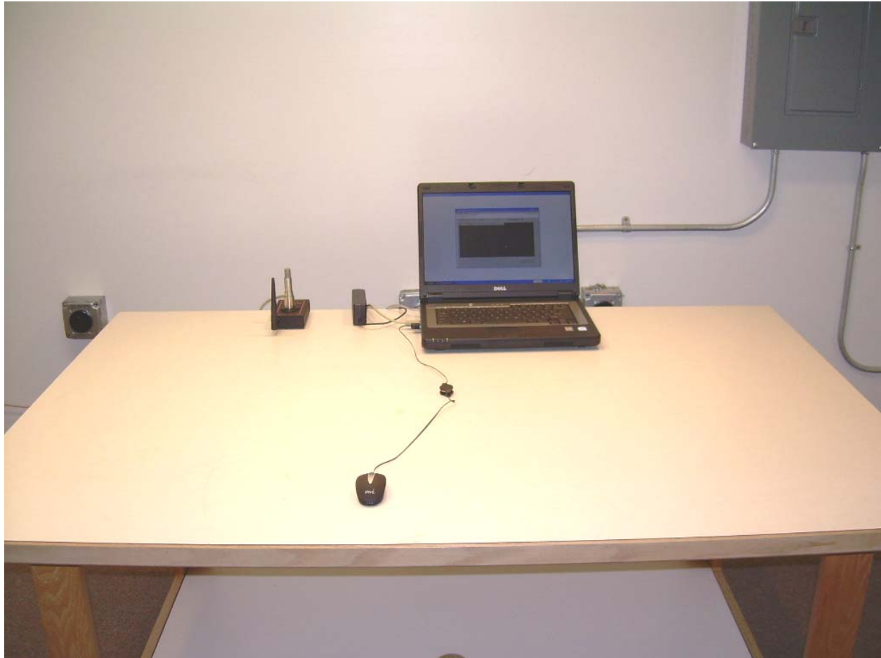
Photograph 3 - Front View Conducted Disturbance Worst Case Configuration
