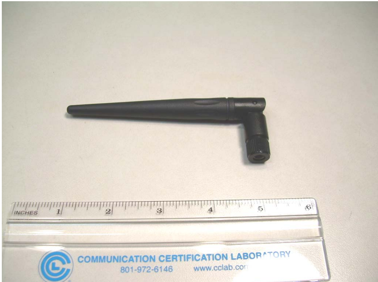
Photograph 11 - View of the MPRF-H Antenna
