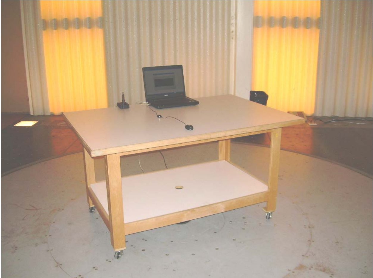
Photograph 1 - Front View Radiated Disturbance Worst Case Configuration
