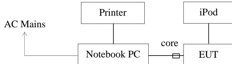
(EUT: FM Transmitter For ipod)
