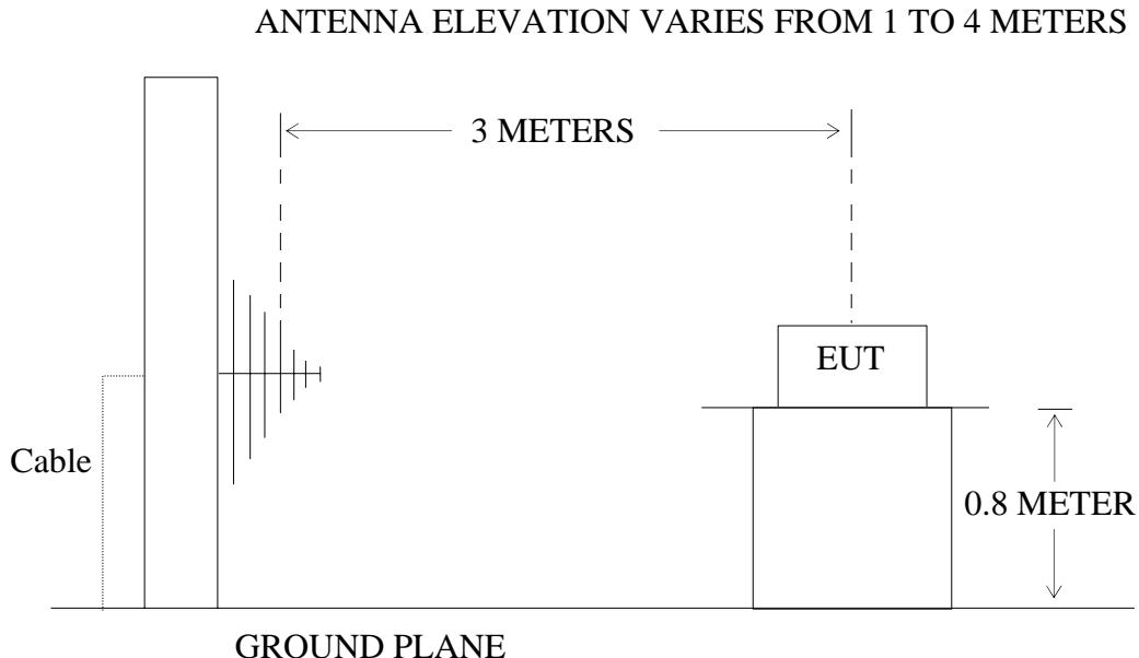
(EUT: FM Transmitter For ipod)
